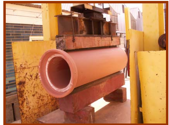
12" VCP 3 Edge Bearing Test
